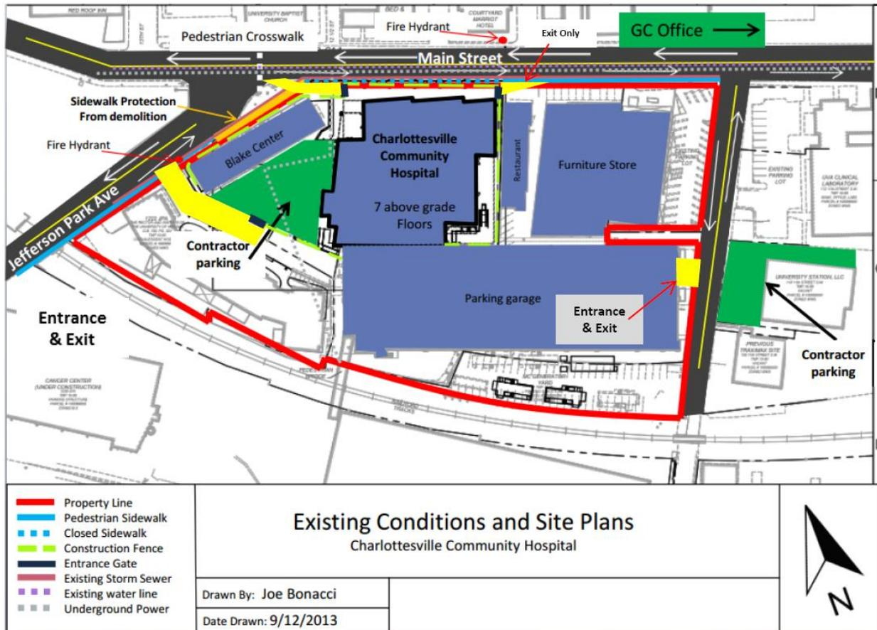
Figure 3; Existing Conditions Site Plan
