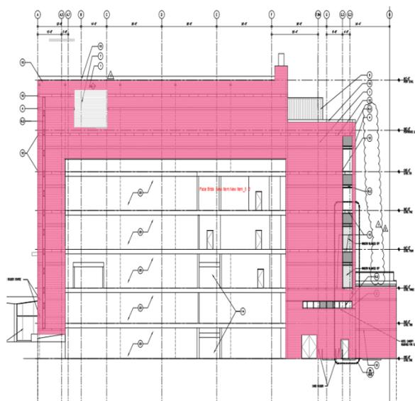
The pink color in each elevation represents the location of all brick veneer with CMU backup. This is also the location where prefabricated panels will be installed. The East wall clearly contains the majority of the material and is the main location of concern for site clutter and safety.
